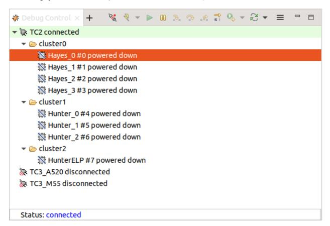
**Note:** This configuration requires Arm DS version 2023.a or later. The names of the cores shown are based on codenames instead of product names. The mapping for the actual names follows the below described convention:
